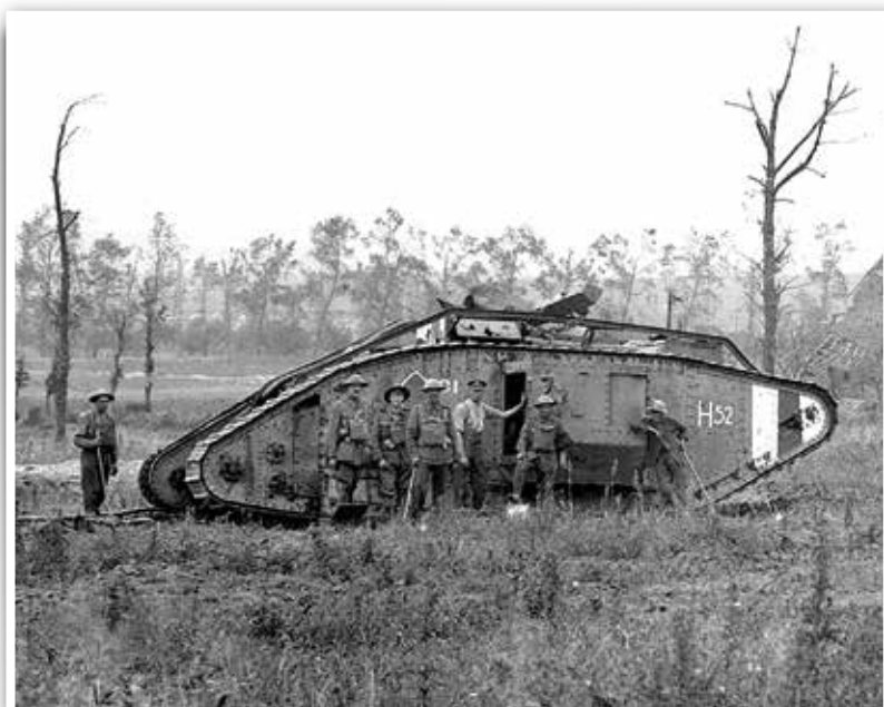
ABOVE Australian soldiers and British tank crew stand beside H52, No. 9001, one of the three Mk. V tanks knocked out of action in the fight for Hamel on 4 July 1918. The left track has been 'thrown' off and the un-ditching beam appears to have been broken. Note the French Tricolour on the roof of the house. It was put there by an officer of 28 th Battalion AIF on the morning of the battle to mark the capture of the position. (Courtesy of the Australian War Memorial; E03843)
